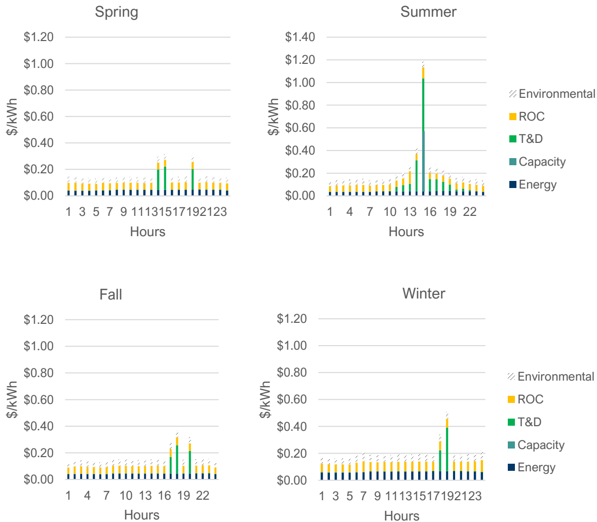
Figure 24. Average Hourly Seasonal Avoided Cost Values for Micro Hydro Facility, Year 2021 Shown (2021$)
